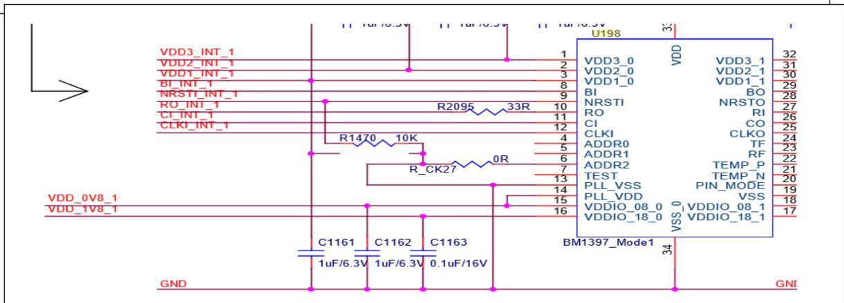
If 0.8V power supply circuit does not have 0.8V output, check if the power supply of 0.8V LDO has about 3.2V power supply voltage. If yes, check whether LDO is in a condition of pseudo soldering/short circuit. If it has 0.8V output, check the resistance to ground of this chip. If the resistance is normal, it should be chip anomaly.
