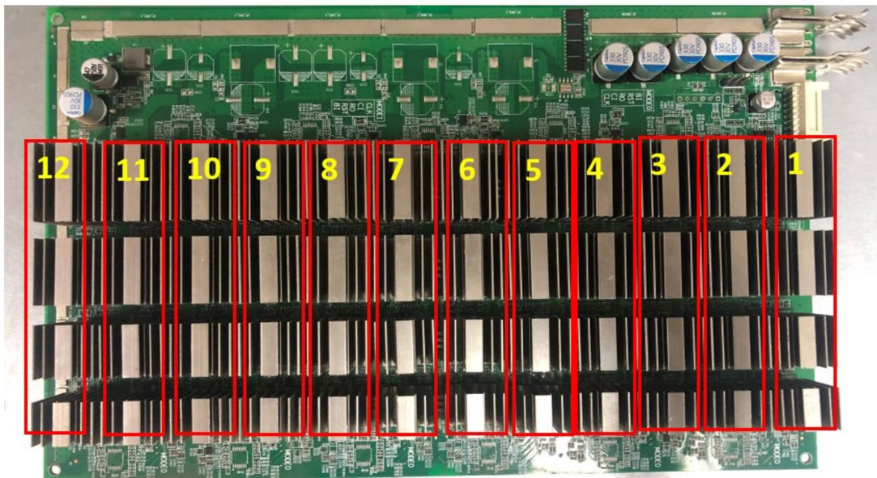
The Distribution and Sequence of Voltage Domain Test Points
