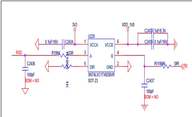
RX and CI Signal and Chip Transfer Schematic Diagram
