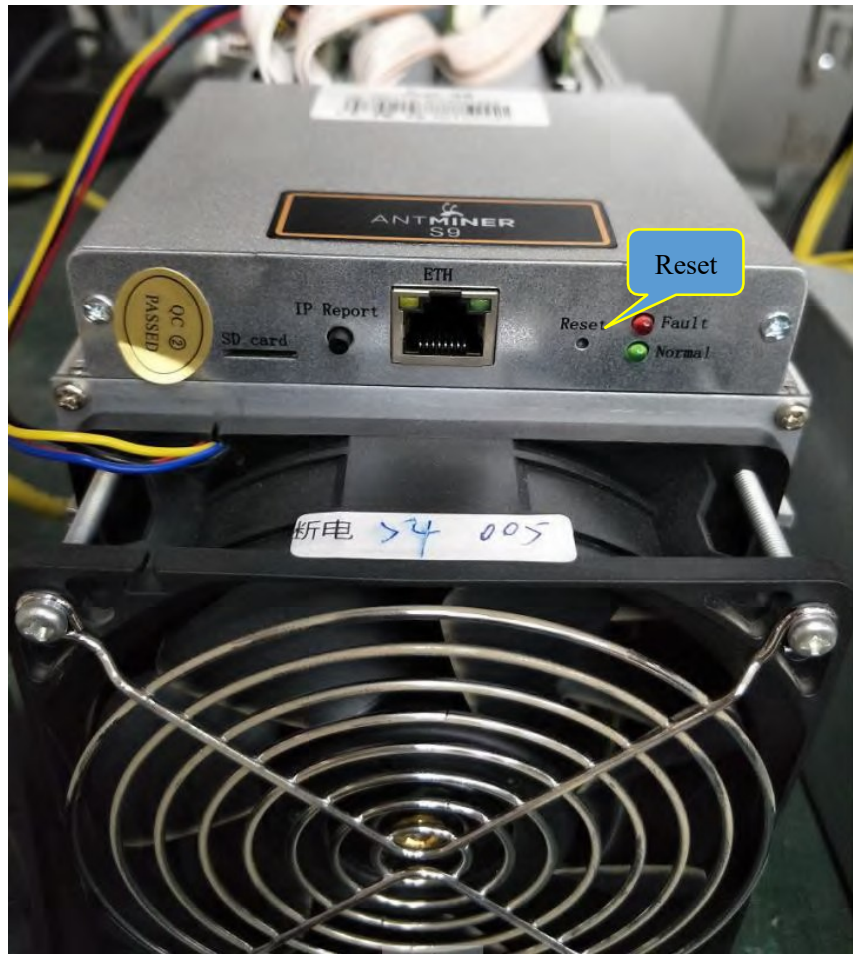
Fig 35. XILINX Control Panel Appearance
