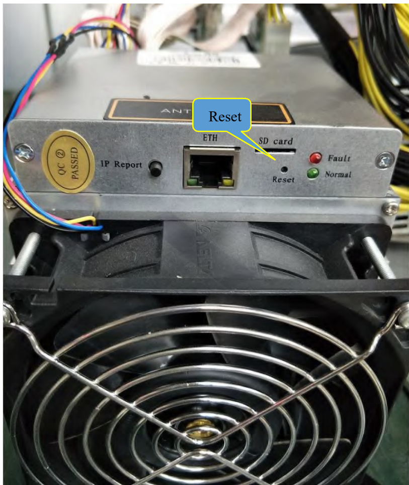
Fig 34. C5 Control Panel Appearance
